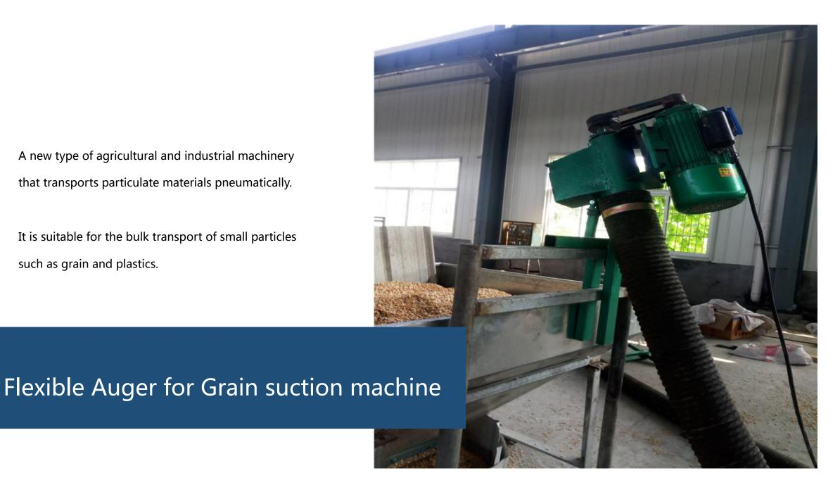
It can be used to transport materials horizontally, inclinedly, and vertically using the layout of the pipe.,
